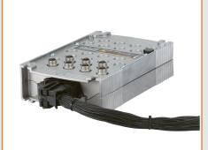
Connection of the I/Os, power supply and references via a lockable central plug with 64 pins of different ampacities.
