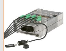
Connection of CAN bus, USB, Ethernet and RS232 via coded, shielded M12 connectors. For convenient access, the USB connector can be incorporated separately in the front panel.
