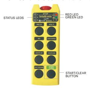
The controls available on the A08 transmitter are largely the same as those on the ICC cab controller. Refer to the section on the ICC for a description of the available commands. The section below describes the special features of the A08 transmitter.
