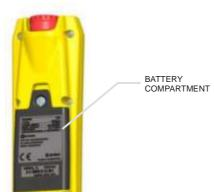
The battery in the A08 transmitter should be replaced when the operating time of the transmitter falls below 8 hours on a single charge.
